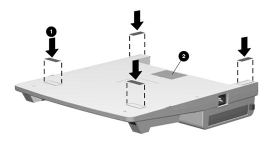
Figure 6-8. Expansion Base Feet and MPEG Connector Door
